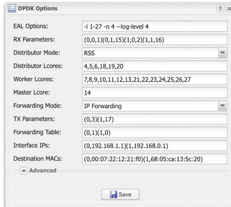
EAL Options contains the parameter “-l 1-27” which configures DPDK to use the lcores 1 to 27 (28 lcores = 14-core CPU with Hyper-threading enabled). The parameter “-n 4” configures DPDK to use 4 memory channels which is the maximum of what the reference Intel Xeon CPU (14-core Broadwell) supports.
