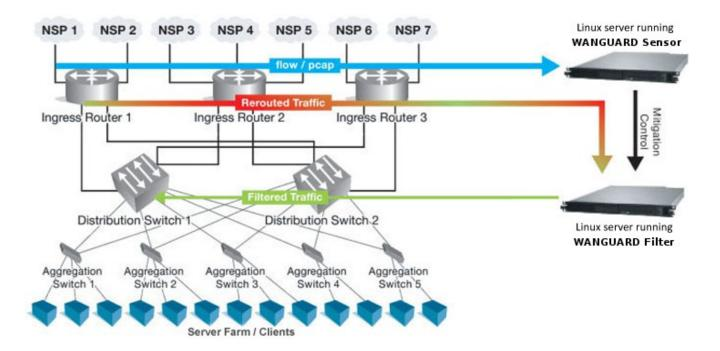
The figure above provides an example of traffic diversion from Ingress Router 1,2,3 towards a Linux server running the Filter software.
