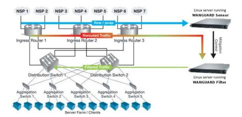
In-line routing – The Filter runs on a server that resides in the main data path, configured as an OSI
