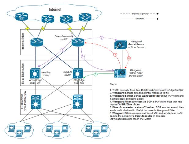
Figure-1. Logical Diagram for an Enterprise Network – how traffic diversion works
