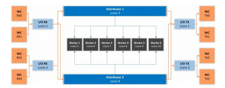
**I/O RX Lcore** performs packet RX from the assigned NIC RX rings and then dispatches the received packets to one or more distributor lcores using RSS or a round-robin algorithm.
