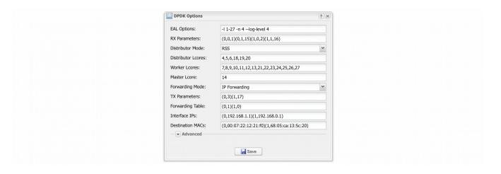
EAL Options contains the parameter "-l 1-27" which configures DPDK to use the lcores 1 to 27 (28 lcores = 14-core CPU with Hyper-threading enabled). The parameter "-n 4" configures DPDK to use 4 memory channels which is the maximum of what the reference Intel Xeon CPU (14-core Broadwell) supports.
