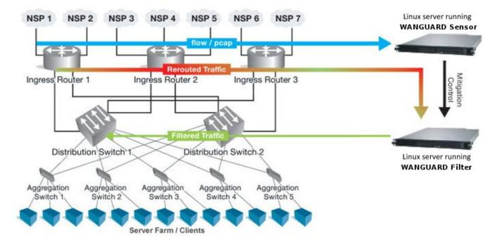
The figure above provides an example of traffic diversion from Ingress Router 1,2,3 to a Linux server running a WANGUARD Filter.
