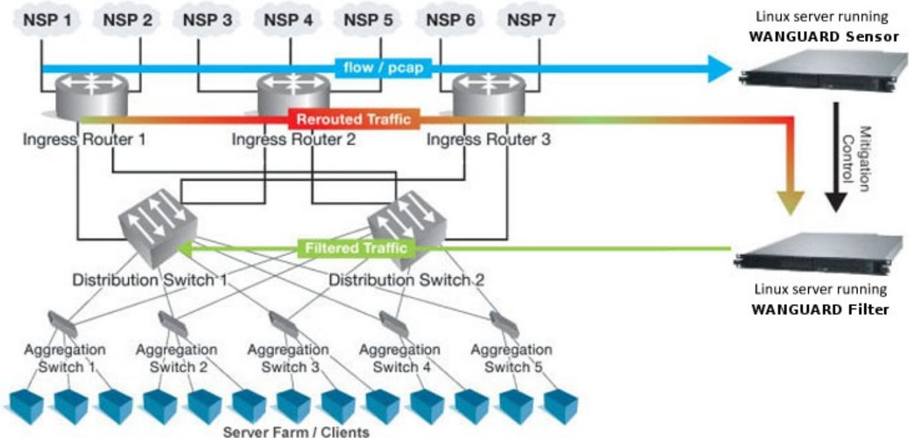
The figure above provides an example of traffic diversion from Ingress Router 1,2,3 towards a Linux server running the Filter software.
