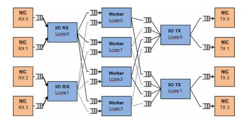
Each **I/O RX Lcore** performs packet RX from its assigned NIC RX rings and then distributes the received packets to the worker threads.
