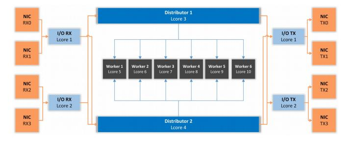
**I/O RX Lcore** performs packet RX from the assigned NIC RX rings and then dispatches the received packets to one or more distributor lcores using RSS or a round-robin algorithm.
